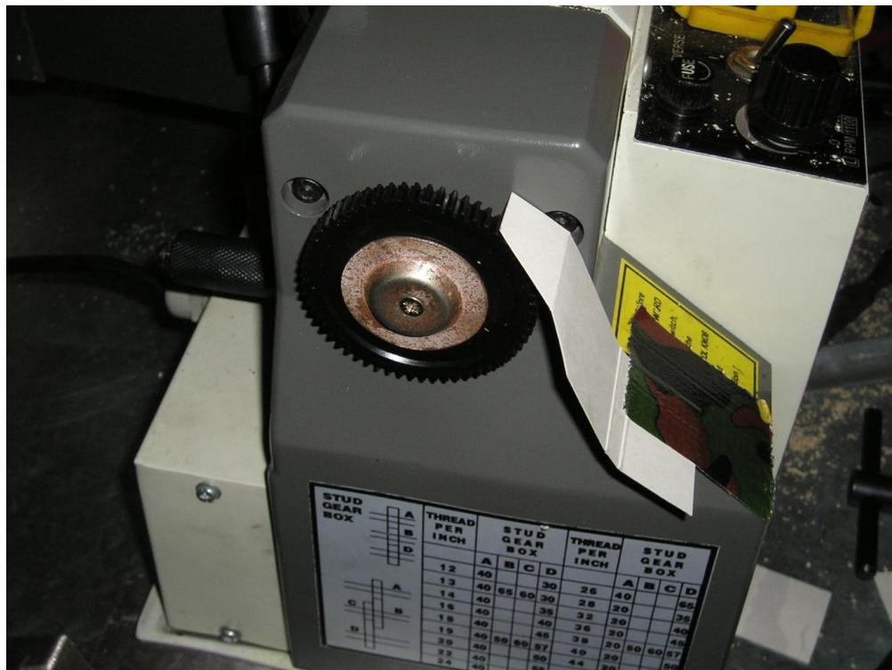
Reassemble the lead screw on the lathe. Adjust the end float .do NOT put the drive gear back on the lead screw. Test for freedom of operation, you possibly will be able to detect errors of bearing alignment that you never noticed previously. Re align bearings as required.
